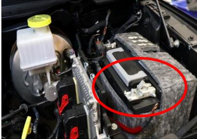
Figure 7- Battery Terminal
