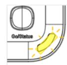
**Flashing Yellow** – Slowly flashing indicates engine running. Fast Flashing indicates POWV3.5 has been activated and providing pre-charge in preparation for a jump-start attempt.
