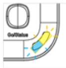
**Alternating Yellow and Blue** - Indicates internal battery is too cold to provide jump-start and the battery heater has been activated. When the battery has reached operational temperatures after a few minutes, the POWV3.5 will be ready to provide a jump-start.
