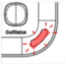
**Blinking Red** – Indicates the POWV3.5 is not ready to be activated because there is a connection error, or the battery is too hot to perform a jump start. The TEMP indicator will also flash red if the battery is too hot.
