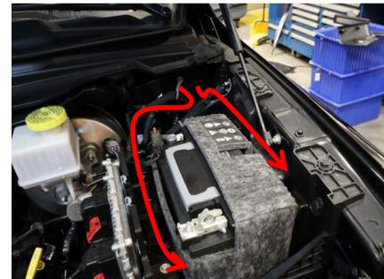
Figure 6- Through Firewall
