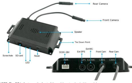
NOTE: The RF Indicator on the front of the unit is not active in this model
