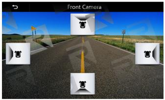
The selected camera will continue to display untill you press the return icon, Media or Home buttons on the radio control panel. If you do not have a camera option such as Rear because you have a factory camera or optional cameras have not been installed no image will appear.
