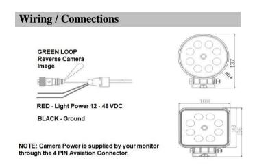
To reverse the camera image, shut off power to the camera, cut the green loop, turn power back on. To restore the image reconnect the green wire. Always tape and seal the cut wire.
