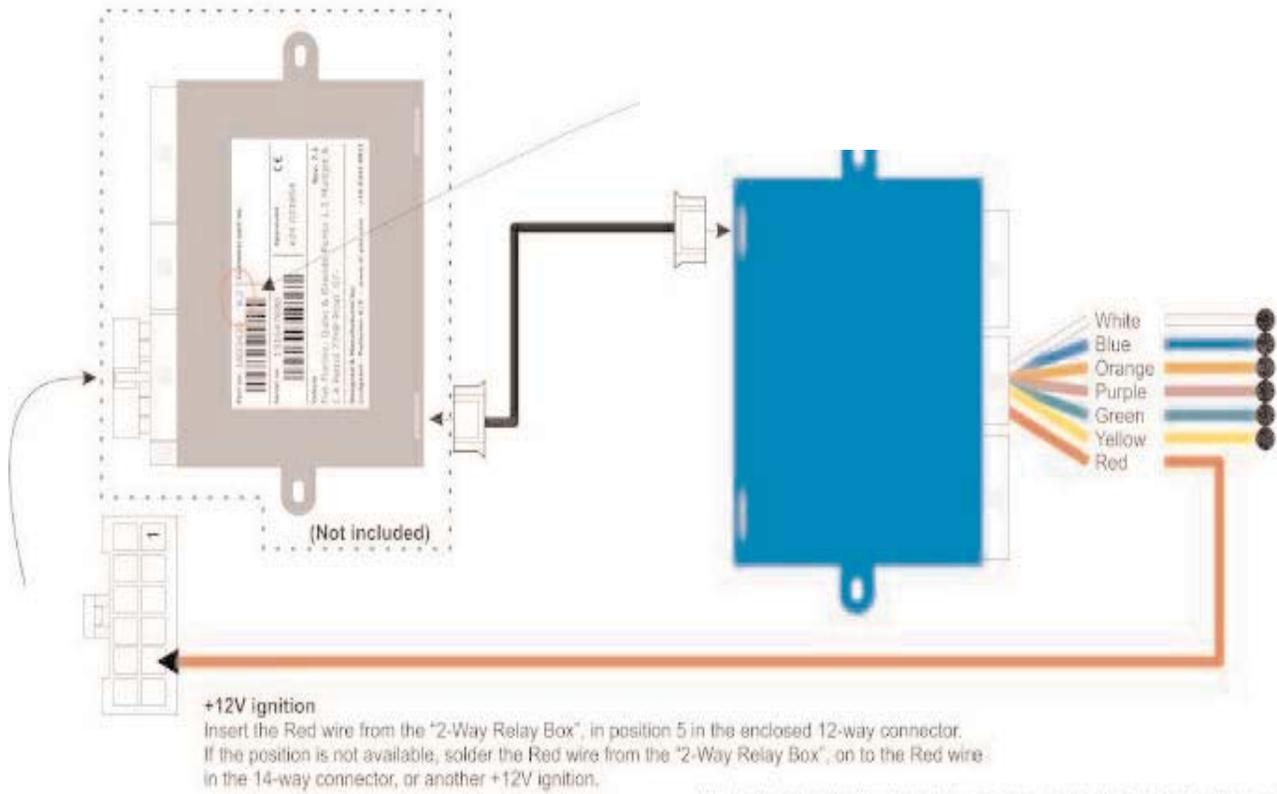
Connect Green wire from 2way relay box to Pos. 2 of the brake switch Orange wire.
