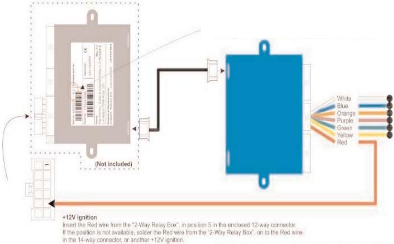
Connect Green wire from 2way relay box to Pos. 2 of the brake switch Red wire.
