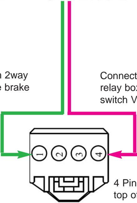
4 Pin Brake switch located at top of brake pedal assembly.
