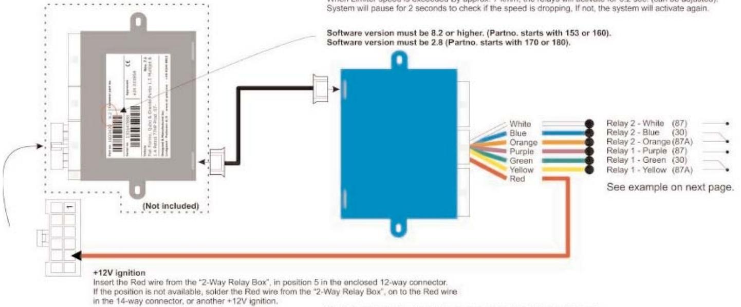
Locate BCM under drivers dash locate Green connector in BCM. Solder 1.9K resistor inline with purple wire from 2way relay box and connect to Positon 9 Green/Brown wire in green connector in BCM. Solder Green wire from 2way relay module to position 4 White/Red wire in green connector of BCM
