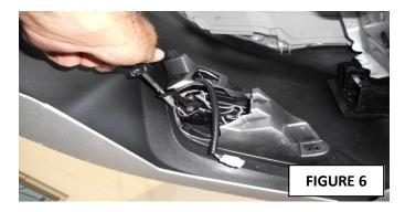
ATTACH TO VEHICLE WITH M5 PHILLIPS HEAD SCREW AS SHOWN IN FIGURE 6.
