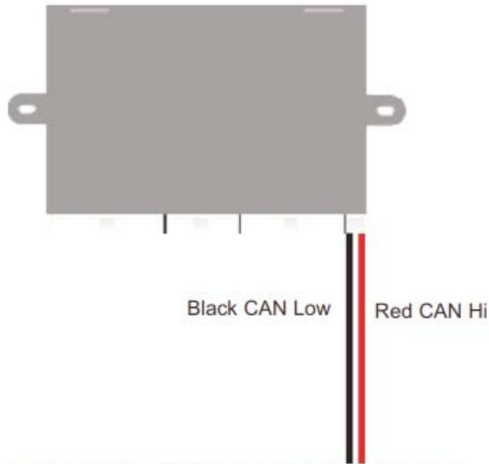
Locate CAN Junction Block behind Headlight Switch on Drivers Dash. Connect Rostra Red CAN high wire to White/Green CAN high wire in White 3 pin connector. Connect Rostra Black CAN low wire to White/Blue wire in White 3 pin connector.
