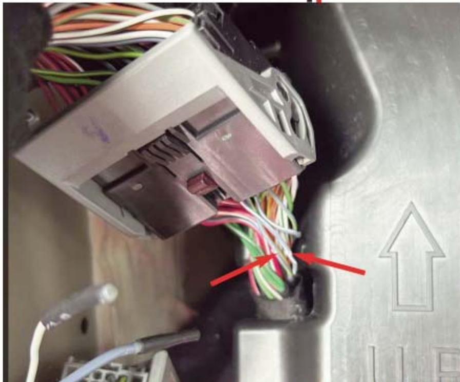
Connect Rostra Red CAN high wire to Blue/White wire in position 7 of Black 48 pin connector behind Drivers Kick panel. Connect Rostra Black CAN low wire to Blue/Yellow wire in position 8 of Black 48 pin connector behind driver kick panel.
