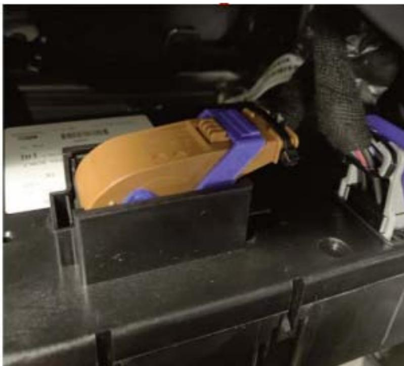
BCM Brown connector in rear of BCM/fuse box 60 pin plug.
