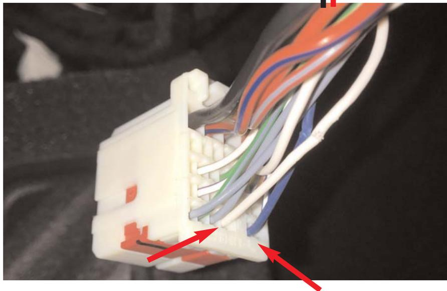
CAN wire connections: Connect Rostra Red CAN high wire to Blue wire in position 25 of White connector in BCM. Connect Rostra CAN low wire to white wire in position 24 of the white connector in BCM.
