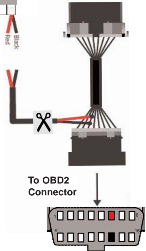
Note: Use a precision tool to press up on the backside of the OBD2 connector housing to release the tab. Push out OBD2 connector toward the back to remove.
