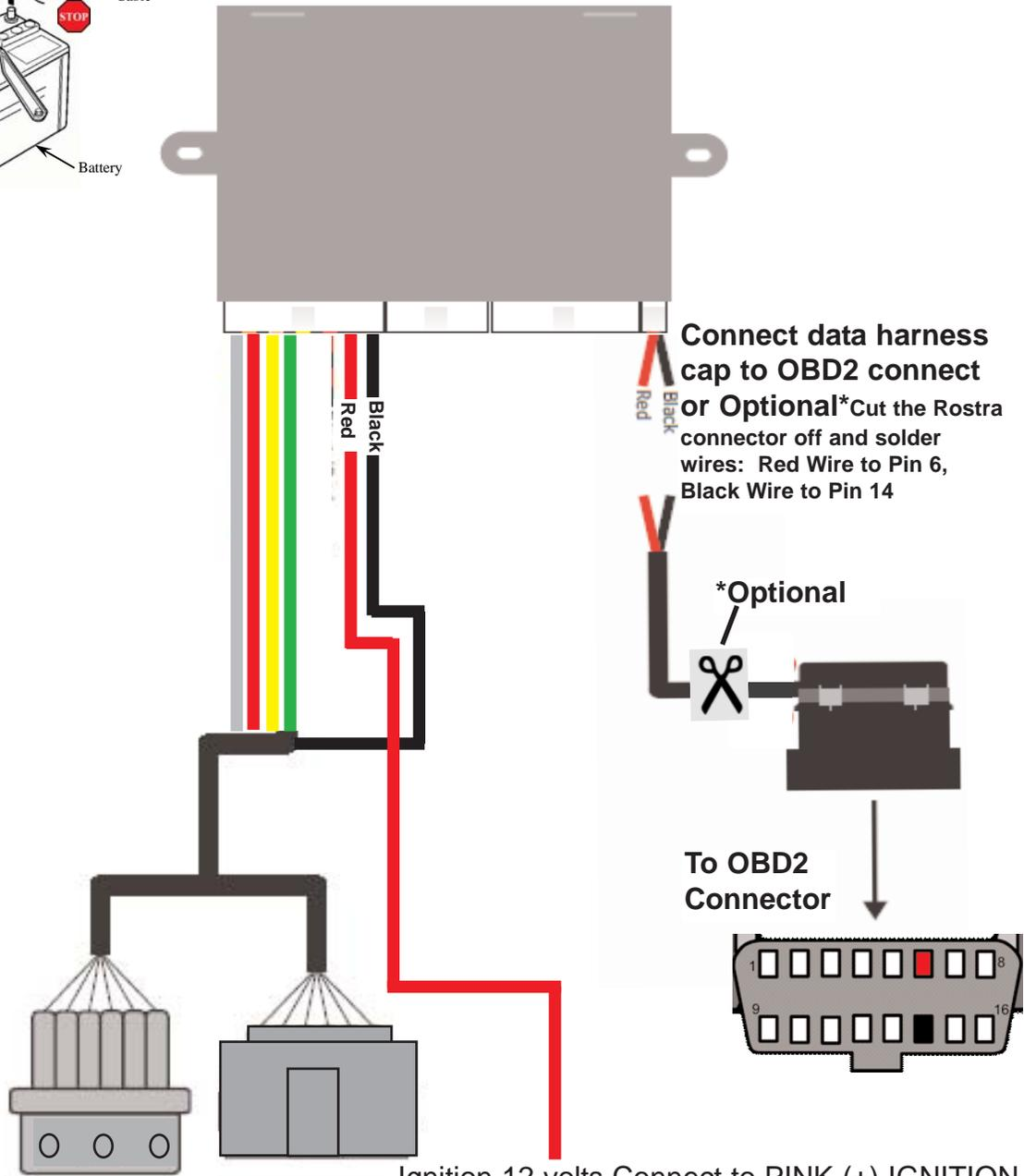
Ignition 12 volts Connect to PINK (+) IGNITION SWITCH OR Pass-thru connector below drivers dash PINK wire shown in figure below.
