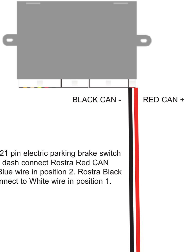
Locate the Gray 21 pin electric parking brake switch under driver side dash connect Rostra Red CAN high wire to the Blue wire in position 2. Rostra Black CAN low wire connect to White wire in position 1.
