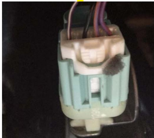
Locate the Brake Switch at top of brake switch assembly. Connect cruise Yellow wire to Violet/White in position 1.
