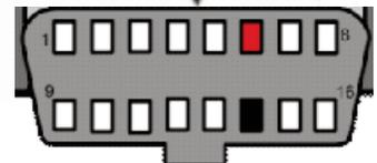
Note: Standard OBD2 Connect Red wire to White/Blue wire in Pin 6 and Connect Black wire to White wire in Pin 14
