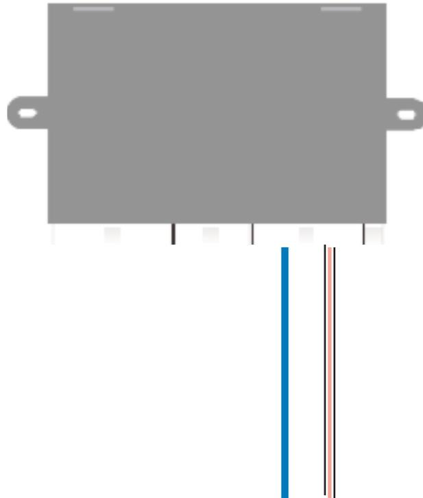
Rostra Blue wire connect to Green/Violet IGNITION power position 5 of the Gray 25 Pin connector in right module of BCM
