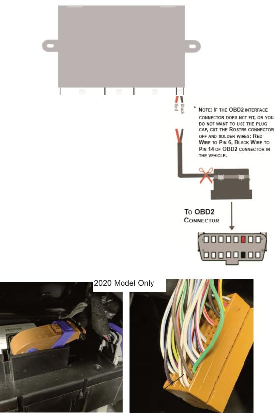
2020 Models CAN wires will need to be soldered to BCM Brown connector in rear of BCM/fuse box. Green wire position 13 CAN positive connect our Red CAN wire. Brown wire position 14 CAN negative connect our Black CAN wire.
