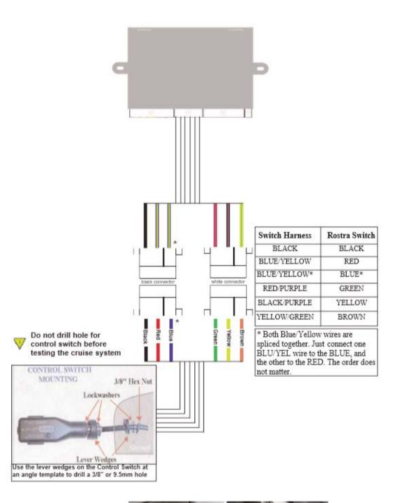
Use the lever wedges on the Control Switch at an angle template to drill a 3/8" or 9.5mm hole
