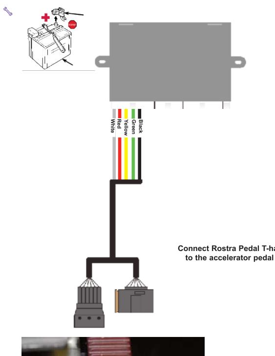
**Connect Rostra Pedal T-harness inline** to the accelerator pedal connector
