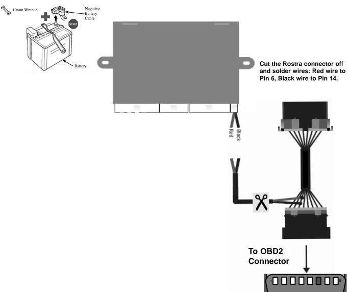
Note: Use a precision tool to press up on the backside of the OBD2 connector housing to release the tab. Push out OBD2 connector toward the back to remove.
