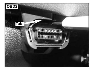
Connect Red wire to White/Blue wire in Pin 6 and Connect Black wire to White wire in Pin 14.
