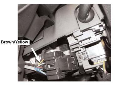
1. Find a suitable position for the switch on the left hand side of the covering around the steering column.
