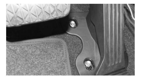
Locate the accelerator pedal as shown in above picture. Remove the 2 10 mm bolts that hold the accelerator pedal to floor board. Once bolts are removed, the pedal assembly will fold out. Continue to next page for accelerator pedal harness instruction.
