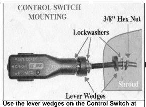
an angle template to drill a 3/8" or 9.5mm hole
