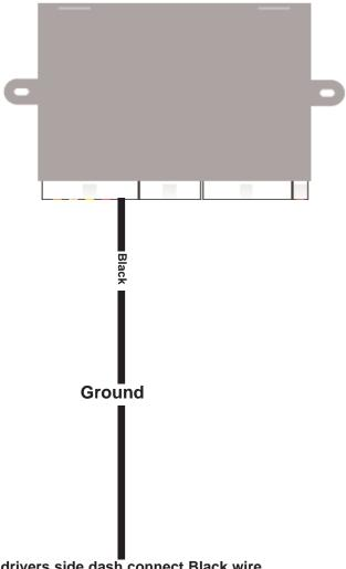
Under drivers side dash connect Black wire ground to factory ground point shown in picture below
