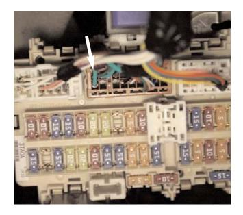
Rogue Under steering column at ignition swicth white 6 pin connector pin position 1 Pink wire connect and solder Red Ignition power
