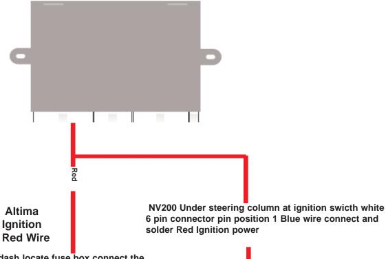
Altima Under Drivers dash locate fuse box connect the Red Ignition power to position 16 Green wire located in the upper middle connector solder connection only
