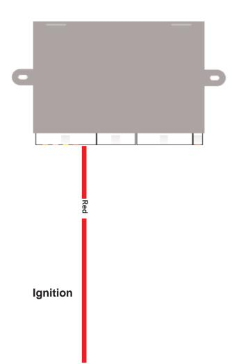
Kia Rio: Connect the Red Ignition wire to pink wire in top left corner of white connector on the left side of the fuse box located under the drivers side dash
