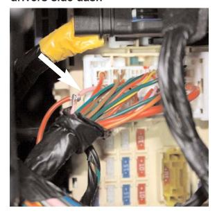
Hyundai Accent: Connect the Red Ignition wire to pink wire in top left corner of white connector on the left side of the fuse box located under the drivers side dash
