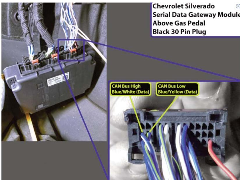
CAN wire connections: Connect Rostra Red CAN high wire to Blue/White wire in position 20 of Serial Data Gateway above accelerator pedal. Connect Rostra Black CAN low wire to Blue/Yellow wire in position 19 of Serial Data Gateway above accelerator pedal.
