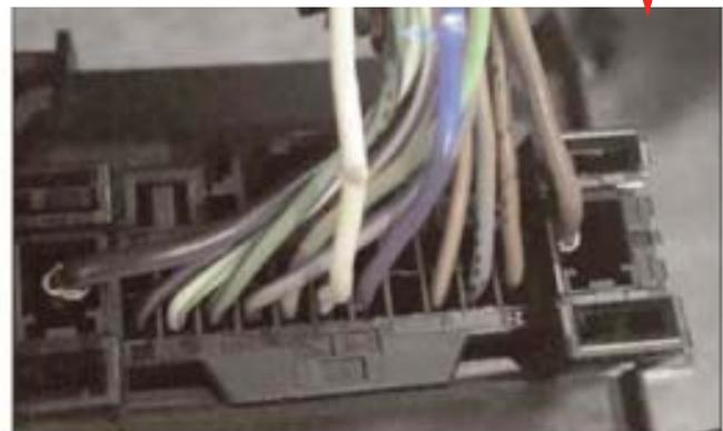
Note: Vehicles Equip. with gateway connector on back of OBD2 solder cruise Red CAN high wire to Blue wire in position 20. Solder Black CAN low wire
