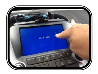
ONCE IN THE NAVI MODE PRESS AND HOLD THE TOUCH SCREEN FOR ABOUT 8 SECONDS UNTIL THE INTERFACE MENU DISPLAYS.
