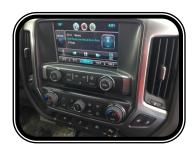
TURN THE IGNIGTION ON, ONCE THE UNIT BOOTS AND THE DISPLAY IS ACTIVE, PRESS AND HOLD THE "HOME" KEY FOR 20 SECONDS UNTIL THE INTERFACE SWITCHES TO NAVI MODE.
