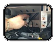
PLUG MOLEX CONNECTOR FROM T-HARNESS INTO THE MAIN HARNESS.
