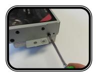
• REMOVE TWO TORX 8 SREWS FROM EACH SIDE, HOLDING THE BRACKETS TO THE SIDE OF THE MONITOR.
