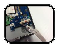
NEXT, PLUG IN CABLE TO PCB IF NOT ALREADY DONE. BE SURE TO PLUG SIDE LABELED "MONITOR SIDE" TO THE PCB. ROUTE THE CABLE OUT THE LOWER CORNER. THERE WILL BE NO NEED TO MODIFY THE CASE AS THERE IS ENOUGH ROOM FOR THE HARNESS TO PASS THROUGH IN THE CORNER.
