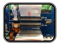
REPLACE FACTORY LCD RIBBON CABLE INTO THE OPEN CONNECTOR ON THE INTRAPHEX PCB. BE SURE TO INSERT IT DEEPLY AND STRAIGHT. PUSH LOCKING TAB DOWN TO LOCK IT IN PLACE.
