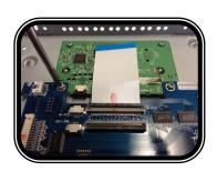
ALIGN INTRAPHEX PROVIDED PCB TO THE TWO HOLES AND REPLACE THE TWO T10 TORX SECURING THE INTRAPHEX PCB.
