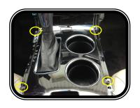
REMOVE FOUR T-20 TORX FROM SHIFTER BEZEL. THERE ARE TWO BESIDE THE "PRNDL" ICONS THAT DO NOT NEED TO BE REMOVED.
