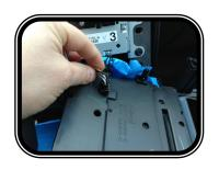
UNPLUG 5 PIN CONNECTOR FROM RADIO FACEPLATE BEZEL.SET RADIO FACEPLATE BEZEL IN A SAFE PLACE TO PREVENT SCRATCHING.
