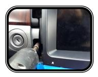
REMOVE FOUR 7MM SCREWS HOLDING RADIO FACE AND LCD FACIA. THEY ARE ONE PIECE. THERE IS NO NEED TO REMOVE THE TWO 7MM SCREWS BESIDE THE AIR VENTS.
