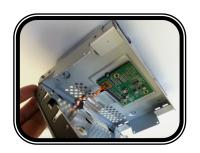
REMOVE LCD, BE CAREFUL WHEN UNPLUGGING THE FFC CABLE AND THE 4 PIN FLAT TOUCH CABLE
