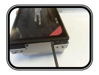
REPLACE THE SCREWS REMOVED EARLIER HOLDING THE LCD.
