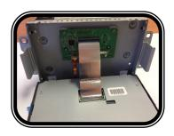
GENTLY OPEN CASE, BE CAREFUL AS THERE ARE RIBBON CABLES CONNECTING THE TWO SIDES.
