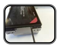
REMOVE TWO #1 PHILLIPS FROM EACH SIDE HOLDING THE LCD.
