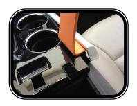
USING A PLASTIC PRY TOOL, PULL UP ON THE TRIM BEZEL FROM THE BACK SIDE RELEASING IT FROM THE CENTER CONSOLE. BE CAREFUL NOT TO SCRATCH THE PIANO BLACK COATING, IT SCRATCHES EASILY.
