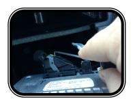
USING A PIC TOOL, PRESS THE RELEASE CLIP TO ALLOW THE LOCKING MECHANISM OF THE MAIN HARNESS TO SLIDE OVER, RELEASING THE PLUG. UNPLUG THE USB.
