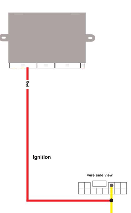
Connect to Yellow wire at White connector to the right of fuse box
