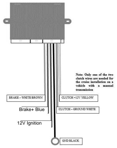
Note: Both brake wires must be connected for cruise to operate. White/Brown must see ground at rest and battery voltage when brake is applied. Blue must see constant battery voltage from brake system.
