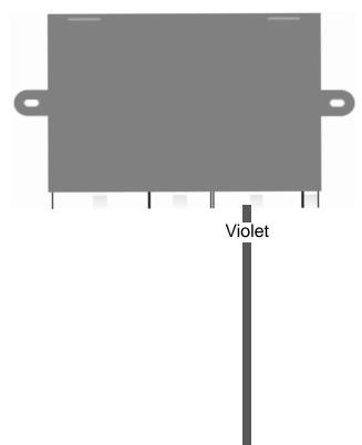
Connect Violet VSS wire to position 3 of the OBD2 connector or if position 3 is bank remove radio locate 24 pin plug in back of head unit position16 White or Yellow wire and solder violet wire connection.
