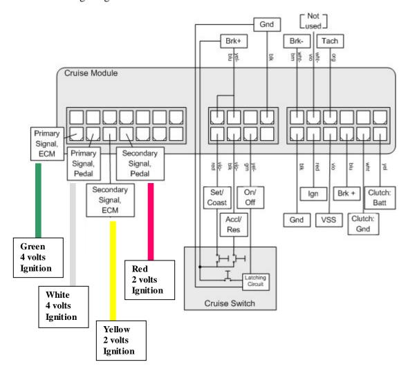
Note: All Pedal Interface Harness Voltages are with pedal fully depressed
