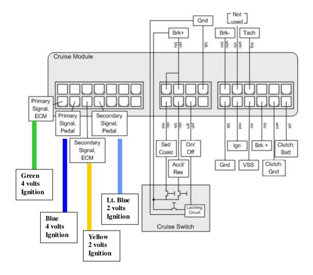
Note: All Pedal Interface Harness Voltages are with pedal fully depressed GM SILVERADO/SIERRA
