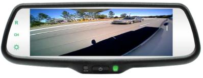
**Auto-Dimming LCD Screen** (available with mirrors 250-8208, 250-8240, 250-8243, and 250-8273)
