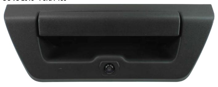
Available with screen interface module for Ford 4.2" display. Part number 250-8419-FDL15 includes module and latch camera.
