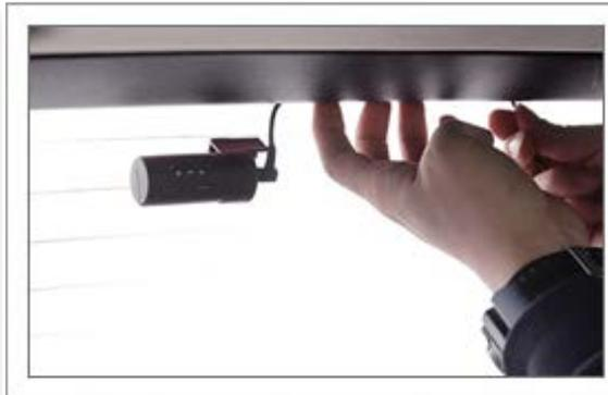
R-cam the cable into window aperture to make it invisible.
