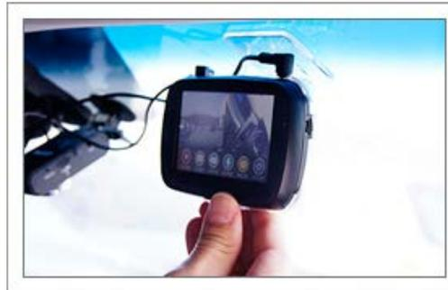
Connect the power cable. There are 2 kinds of power cable - hardwire power cable and cigar power cable..
