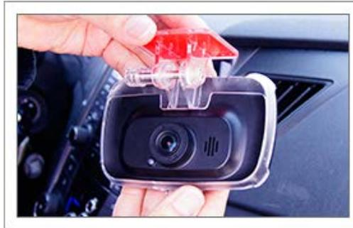
Keep mount holder securely locked in the main unit. Fix the middle latch of holder on the slit above lens of the main camera first. Then fix lower part of holder until hearing clicking sound.
