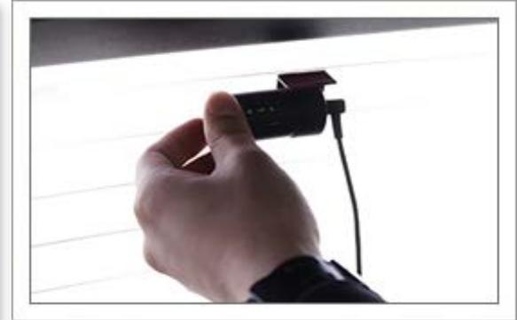
Adjust camera angle with angle adjustor.
