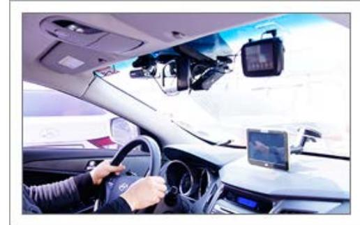
After booting, you can see front and rear video on the LCD screen. Check if it records well and adjust camera angle if necessary.
