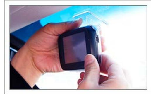
In order to avoid affecting driver's sight, it's better to choose a space in the back of room mirror, than fix the mount holder into it securely by enclosed double-sided tape.
