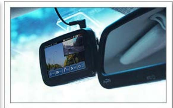
Check the rear cam view after starting engine.
