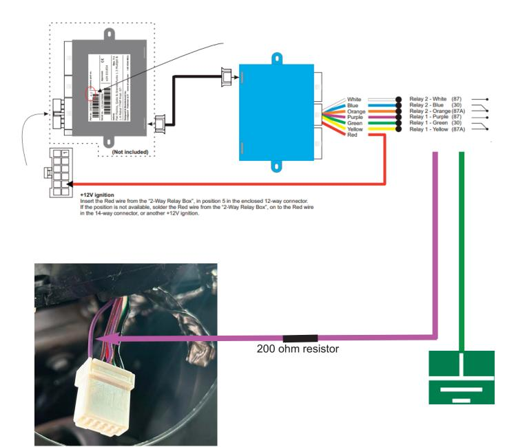
Locate Clock Spring 6 pin connector under steering column. Place 200 ohm resistor in series with Purple wire from 2way relay module and connect to position 6 Violet wire signal 1 OEM cruise input. Connect Green wire from 2way relay module to ground.
