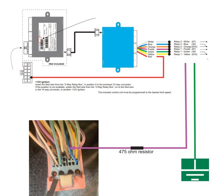
Locate the BCM under driver side dash area. Locate far right section BCM block 2X Pink 32 pin connector. Place in series 475 ohm resistor with Purple wire from 2way relay module and connect to postion 14 Brown/Green OEM cruise input. Connect Green wire from 2way relay module to ground.
