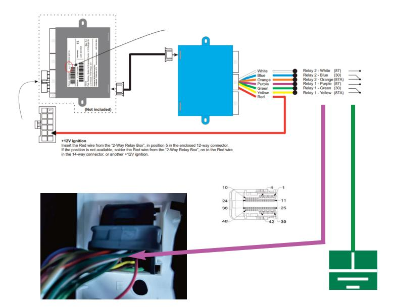
Locate Black 48 pin connector at BCM under drivers dash panel. Connect Violet wire from 2way relay module to Green/White wire in position 11 parking brake sense wire.Connect Green wire from 2way relay module to ground.
