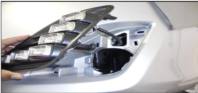
**PASS DRLS THROUGH OPENING AS SHOWN IN FIGURE 3 AND FIGURE 4.**
