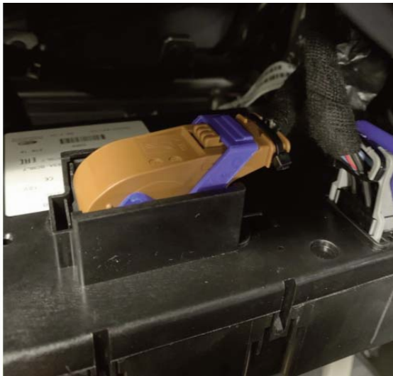
BCM Brown connector in rear of BCM/Fuse box 60 pin plug. Green wire position 52 CAN positive connect Rostra Red CAN wire. Brown wire position 53 CAN negative connect Rostra Black CAN wire.
