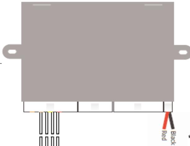
\* NOTE: IF THE OBD2 INTERFACE CONNECTOR DOES NOT FIT, OR YOU DO NOT WANT TO USE THE PLUG CAP, CUT THE ROSTRA CONNECTOR OFF AND SOLDER WIRES: RED WIRE TO PIN 6, BLACK WIRE TO PIN 14 OF OBD2 CONNECTOR IN THE VEHICLE.
