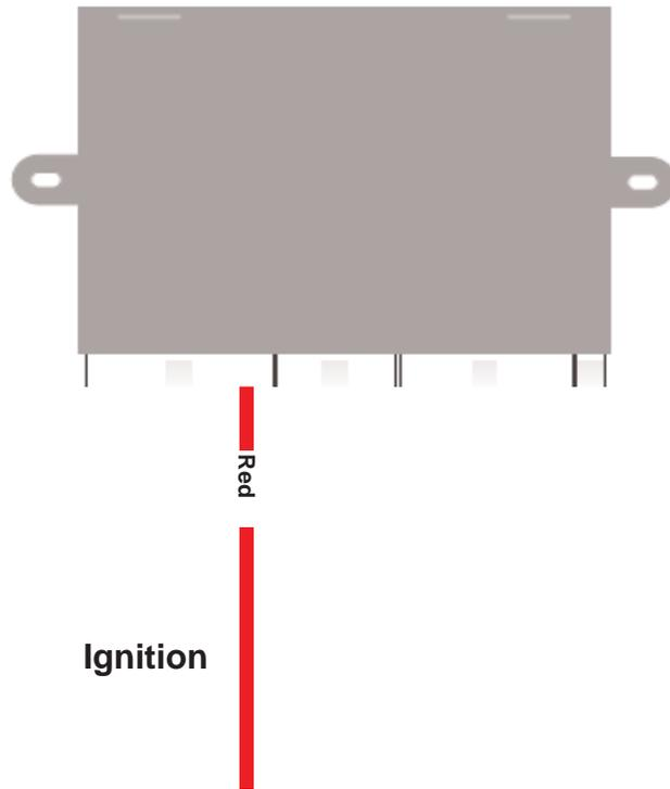
Check ignition wire with a volt-meter to be sure voltage is 0V with key off and holds at +10V during crank/start
