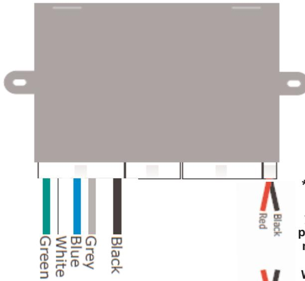
**\*Note:** If the OBD2 interface connector does not fit, or you do not want to use the plug cap, cut the Rostra connector off and solder wires: Red Wire to Pin 6, Black Wire to Pin 14 of OBD2 connector in the vehicle.
