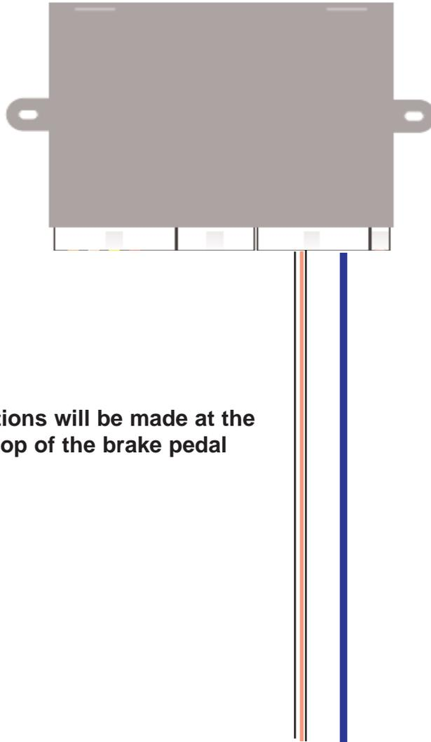
**Note: Brake connections will be made at the brake switch at the top of the brake pedal assembly**
