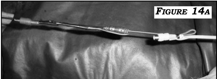
SEPARATE LEADS OF HARNESS TO PULL THROUGH HOSE GROMMET; USE SOAPY WATER LUBRICANT
