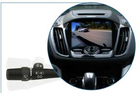
Turn Signal-Activated Side-View Cameras Side-view cameras integrated into the vehicle's mirrors can easily display video from the vehicle's blindspots when the left or right turn signals are active. Blindspot cameras can also be powered on manually via the touch screen's Camera icon.
