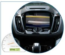
Speed-Controlled Forward Camera A front-facing camera can be triggered to power on automatically when the vehicle is in motion at less than 10 MPH or manually with a long press of the momentary button included with each system.
