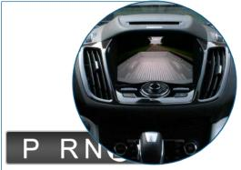
Reverse-Triggered Bed-View Camera Real-time monitoring of the bed or cargo area of the vehicle can be achieved using the selectable reverse camera option to display video while on the road or when the vehicle is placed in reverse - an ideal solution for fifth-wheel trailer connectivity.
