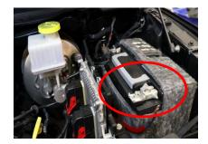
Figure 7- Battery Terminal
