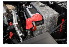
Figure 9- Ground Lug Connection
