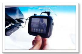
Connect the power cable. There are 2kinds of power cable - hardwire power cable and cigar power cable...
