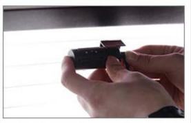
Connect the rear camera cable into the rear camera. (some cameras have already cable fixed)
