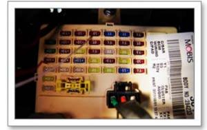
Connect ACC and BATT into fuse. Refer to the hardwire power cable Guide to check the location.
