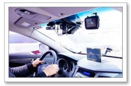
After booting, you can see front and rear video on the LCD screen. Check if it records well and adjust camera angle if necessary.
