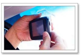
In order to avoid affecting driver's sight, it's better to choose a space in the back of room mirror, than fix the mount holder into it securely by enclosed double-sided tape.
