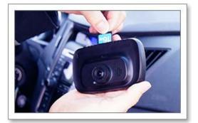
Insert a SD card before using the device. (Micro SD card is already inserted in the device)
