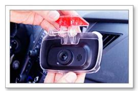
Keep mount holder securely locked in the main unit. Fix the middle latch of holder on the slit above lens of the main camera first. Then fix lower part of holder until hearing clicking sound.
