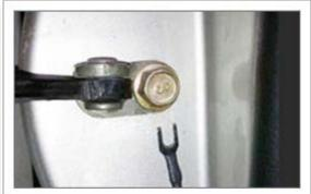
Fix the GND on the nut connected in metal in the car.
