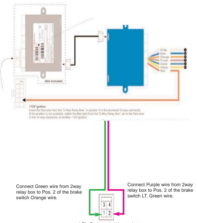
4 Pin Brake switch located at top of brake pedal assembly.
