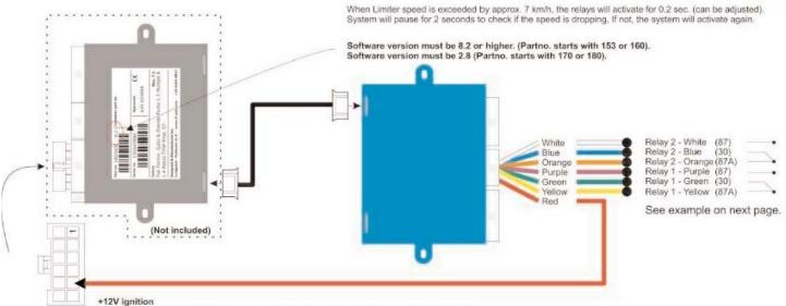
Insert the Red wire from the "2-Way Relay Box", in position 5 in the enclosed 12-way connector. If the position is not available, solder the Red wire from the "2-Way Relay Box", on to the Red wire in the 14-way connector, or another +12V ignition.
