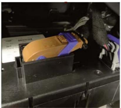
BCM Brown connector in rear of BCM/fuse box 60 pin plug. Rostra Red ignition wire connect to DK. Blue wire in position 12.
