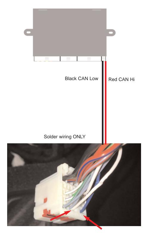
CAN wire connections: Connect Rostra Red CAN high wire to Blue wire in position 25 of White connector in BCM. Connect Rostra CAN low wire to white wire in position 24 of the white connector in BCM.
