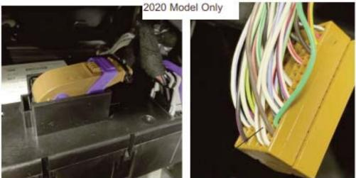
2020 Models CAN wires will need to be soldered to BCM Brown connector in rear of BCM/fuse box. Green wire position 13 CAN positive connect our Red CAN wire. Brown wire position 14 CAN negative connect our Black CAN wire.
