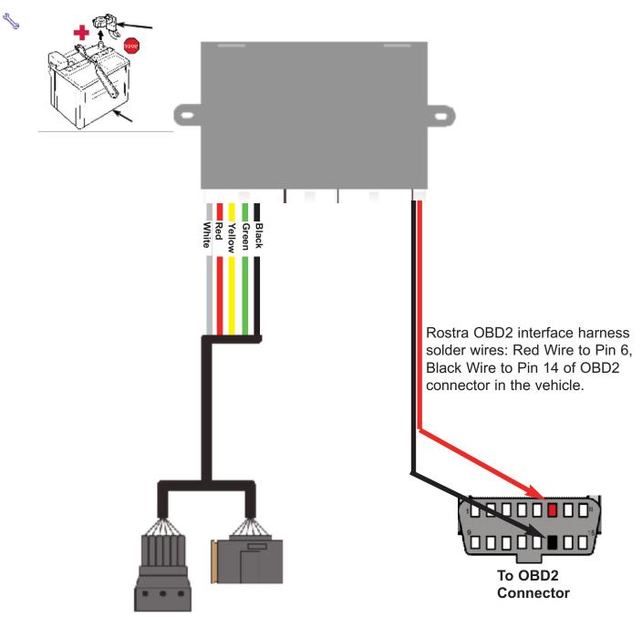
Unplug factory acelerator connector and connect Rostra pedal harness in series
