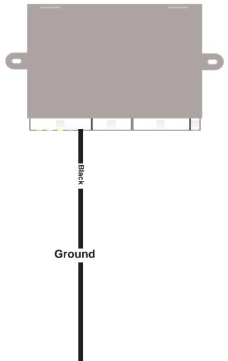
Under drivers side dash connect Black wire ground to factory ground point shown in picture below
