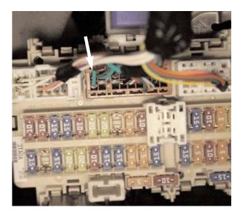
Rogue Under steering column at ignition switch white 6 pin connector pin position 1 Pink wire connect and solder Red Ignition power
