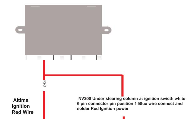
Altima Under Drivers dash locate fuse box connect the Red Ignition power to position 16 Green wire located in the upper middle connector solder connection only
